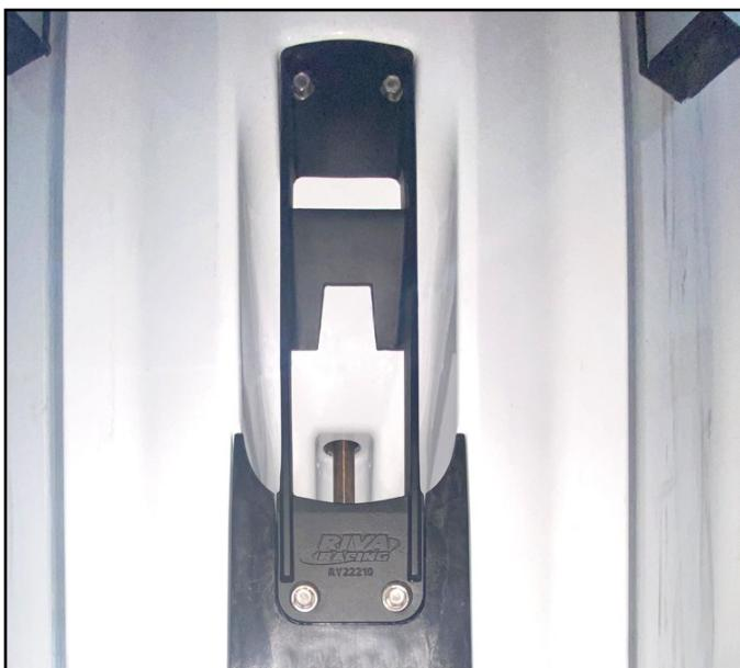
**NOTE: Apply blue Loctite 242 to bolts. Torque bolts to 13 ft•lb (17 N•m). DO NOT USE IMPACT TOOLS!**
